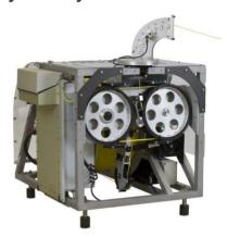
Winch options available including automatic tension control for the fibre optic winch.
