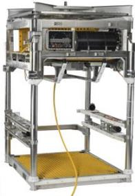
Tether Management System (TMS) Type 8 allowing for the deployment of the vehicle at working depth and also providing protection.
