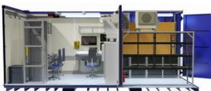
Safe Area 20ft split Control Cabin with a Pilot Control section and a separate high voltage PSU section. Fitted with electric power distribution panels, lighting, air conditioning, heating and 19 inch racks. An optional installed escape hatch is available as is a Zone II upgrade.
