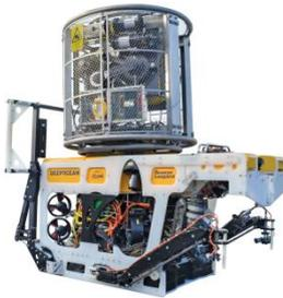
Top Hat style Tether Management System with a 400 m winch module for a 20 mm tether fitted with latch status and line out sensors. Options include lights and cameras.
