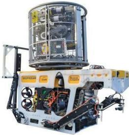
Top Hat Tether Management System with 350m capacity of 20mm tether, fitted with latch status and line out sensors. Options include depth and current sensors, and additional downward looking light and camera.
